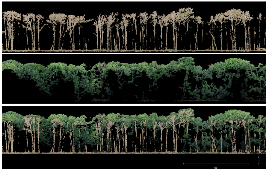
Figure 1: A profile cross-section of the normalized point clouds from the study area in Hainich National Park was created using UAV RGB images and an structure from motion (SfM) approach. The top section displays the point cloud without leaves from March 29, 2022, the middle section shows the point cloud with leaves from August 4, 2021, and the bottom section presents a merged dataset combining both.
